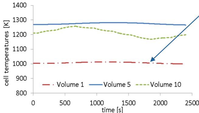
Air temperature effects outlet temp but not inlet. Relatively thick cathode (1 mm) insulates the anode inlet.
