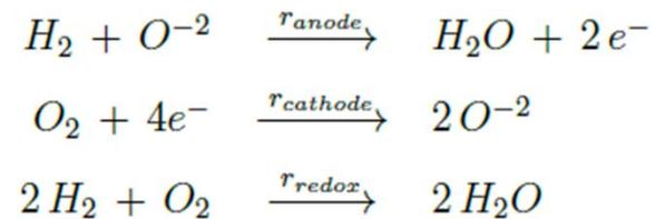
Electricity is primarily produced through H<sub>2</sub> oxidation. CO oxidation also occurs.
