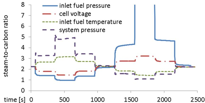
Adding fuel (increasing pressure or decreasing temperature) causes the steam-to-carbon ratio to decrease.
