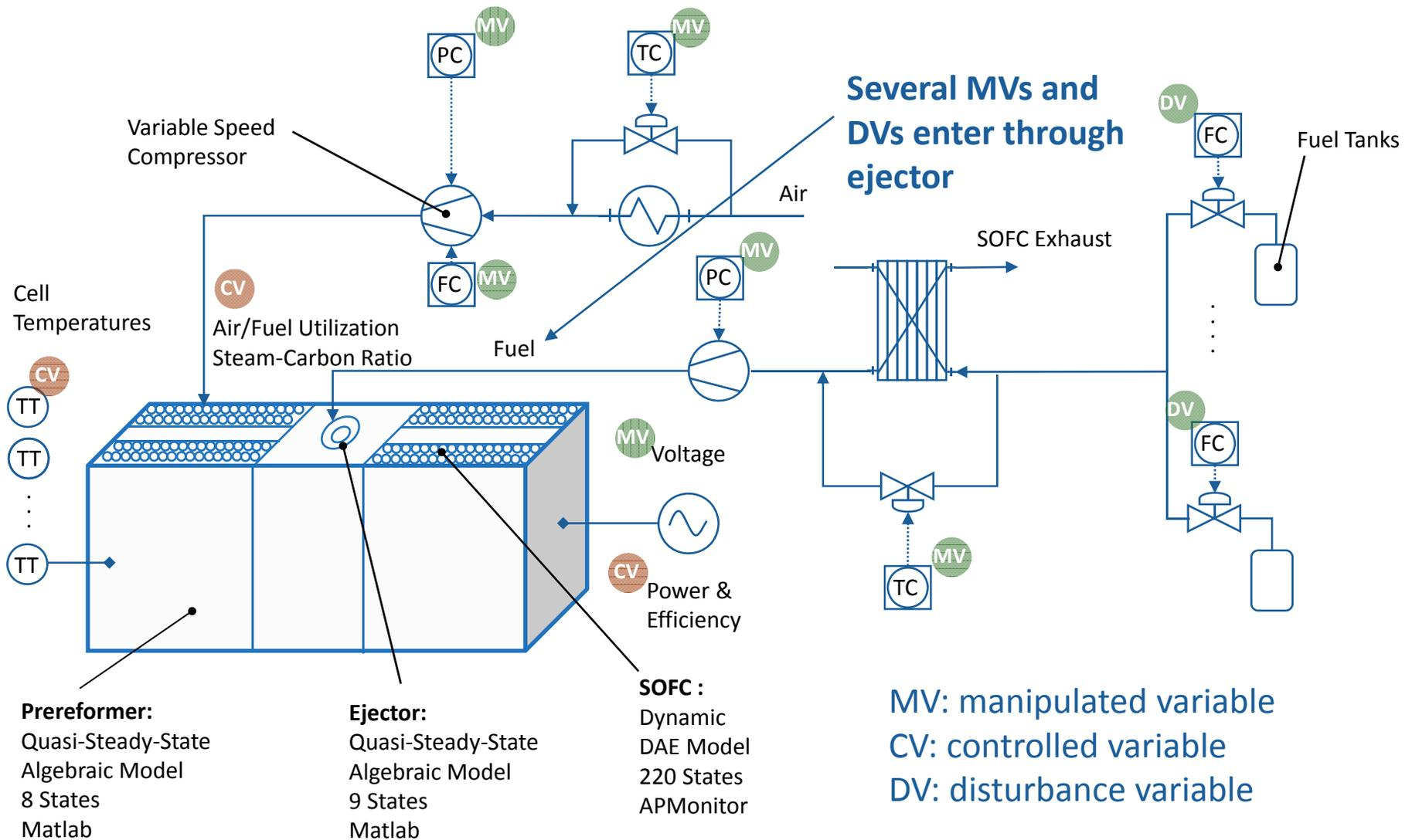
Ejector and prereformer models are necessary to accommodate realistic MVs
