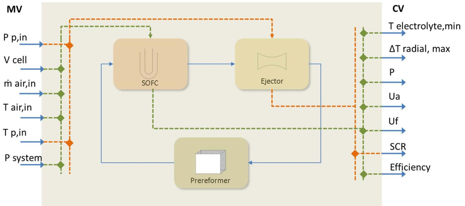
SOFC, ejector, and prereformer models are solved at each time step to investigate MV-CV relationships
