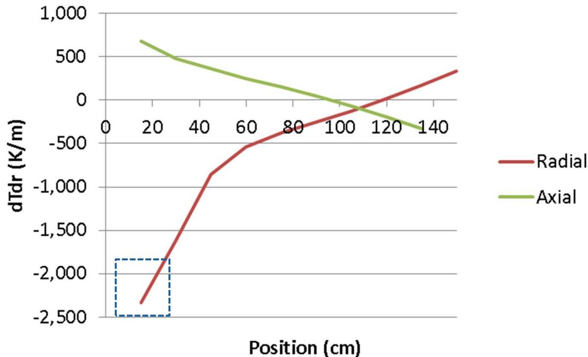
Simulation results agree with prior studies indicating that radial thermal gradients are most significant.
