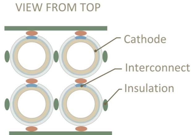
Tubular cells are arranged in bundles and connected in series.
