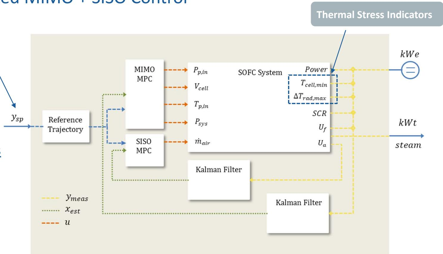
Measurements or estimates of the thermal stress indicators are used directly as controlled variables.
