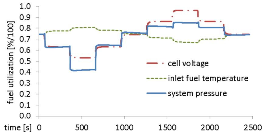
Voltage has linear effect on fuel utilization – voltage changes current directly, thereby changing fuel consumption.
