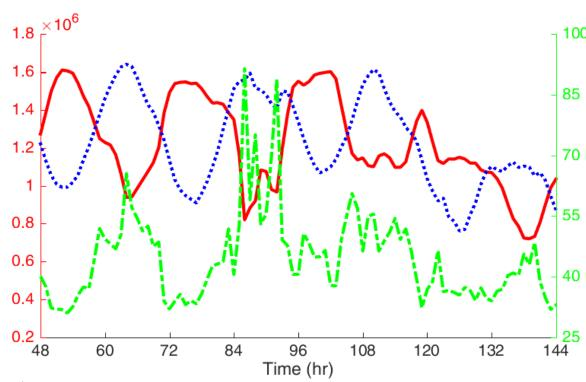
➤ Reduction in CO<sub>2</sub> stripping load during periods with expensive electricity price and increase in stripping load when electricity is cheap
