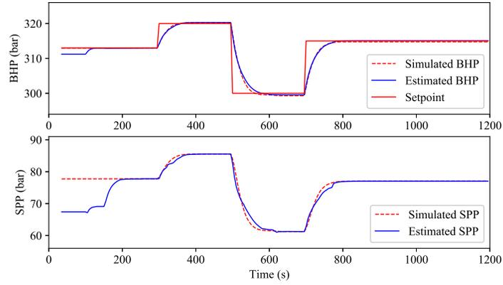
(a) Bottomhole pressure (CV) and Standpipe pressure
