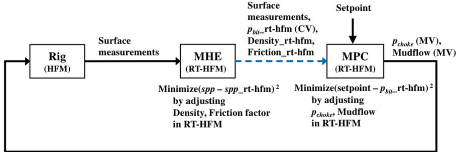
Figure 4: Semi-Closed loop control configuration - Bottomhole pressure is estimated by Moving horizon estimator
