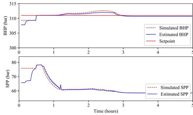
(a) Bottomhole pressure (CV) and Standpipe pressure
