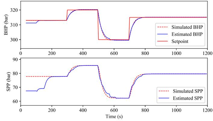
(a) Bottomhole pressure (CV) and Standpipe pressure
