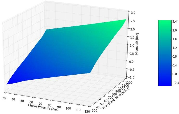
Figure 3: Difference between steady state BHP output from HFM and RT-HFM to identify model mismatch at varying conditions
