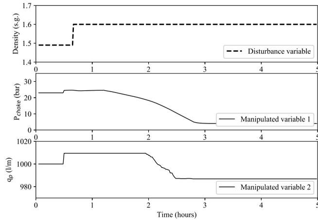
(c) Choke pressure (MV) and Mud flowrate (DV)
