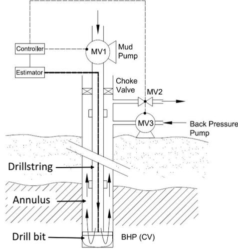
Figure 2: MPD Schematic
