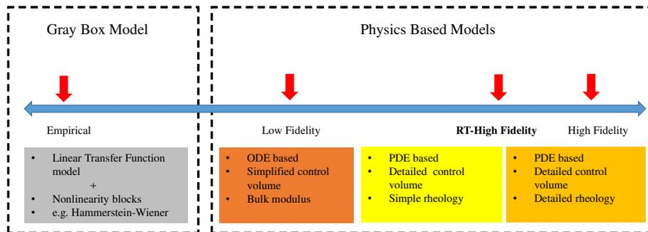
Figure 1: Spectrum of model fidelity in MPD automation
