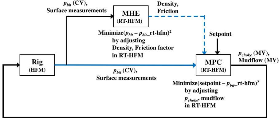
Figure 5: Full-Closed loop control configuration - Bottomhole pressure is directly measured and transmitted by bottomhole sensor and high speed telemetry. Friction factors are estimated for MPC model calibration
