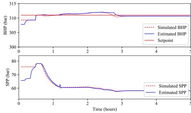
(a) Bottomhole pressure (CV) and Standpipe pressure
