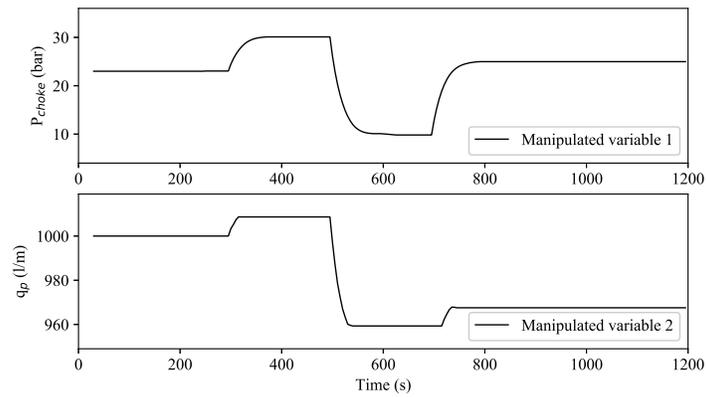
(c) Choke pressure (MV1) and Mud flowrate (MV2)
