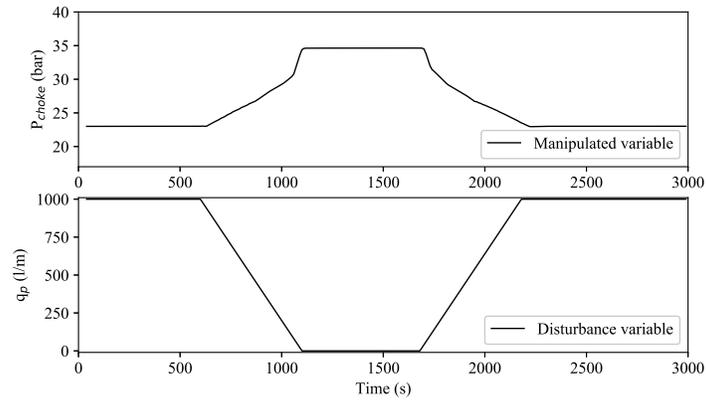
(c) Choke pressure (MV) and Mud flowrate (DV)
