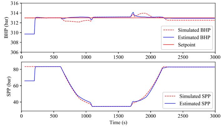
(a) Bottomhole pressure (CV) and Standpipe pressure
