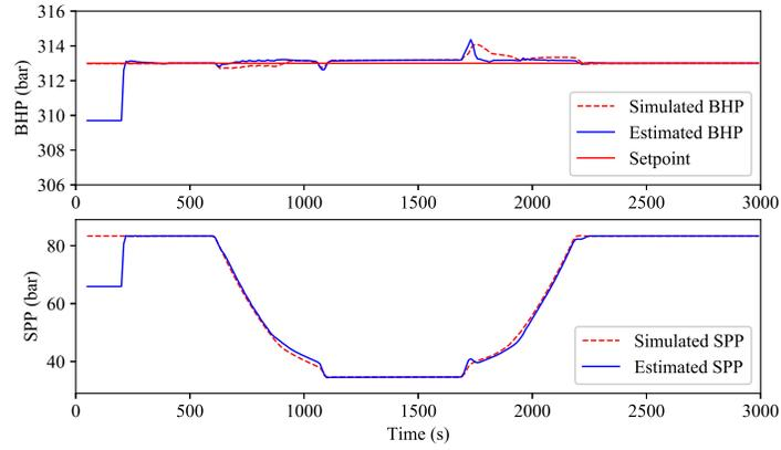
(a) Bottomhole pressure (CV) and Standpipe pressure
