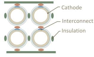
Tubular cells are arranged in bundles and connected in series.
