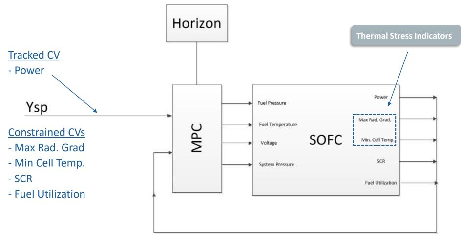
Measurements or estimates of the thermal stress indicators are used directly as controlled variables.
