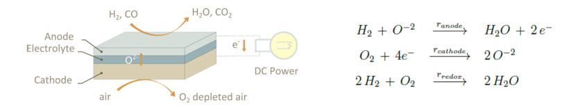
Electricity is primarily produced through H<sub>2</sub> oxidation. CO oxidation also occurs.
