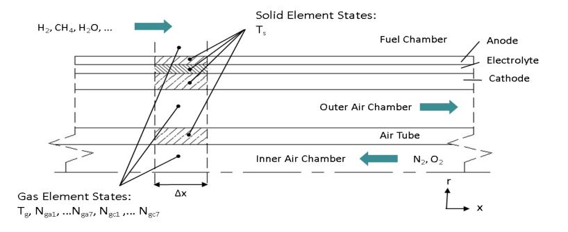
Temperatures, Molar Flows, Current, and Intermediate Variables calculated for each radial element for both dynamic and steady state operation.
