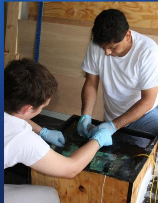
Adhesive Clamp Installation on 8-inch Test Pipe
