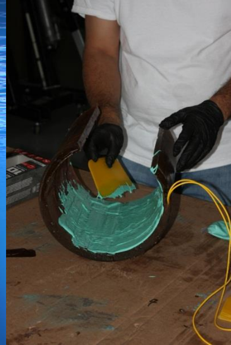
Adhesive Clamp Installation on 8-inch Test Pipe
