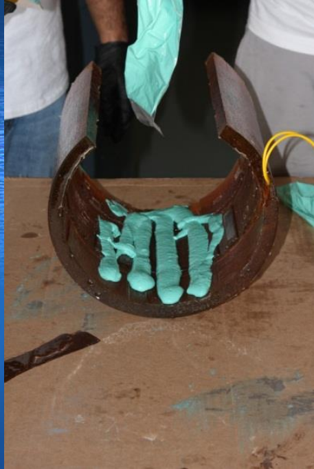
Adhesive Clamp Installation on 8-inch Test Pipe
