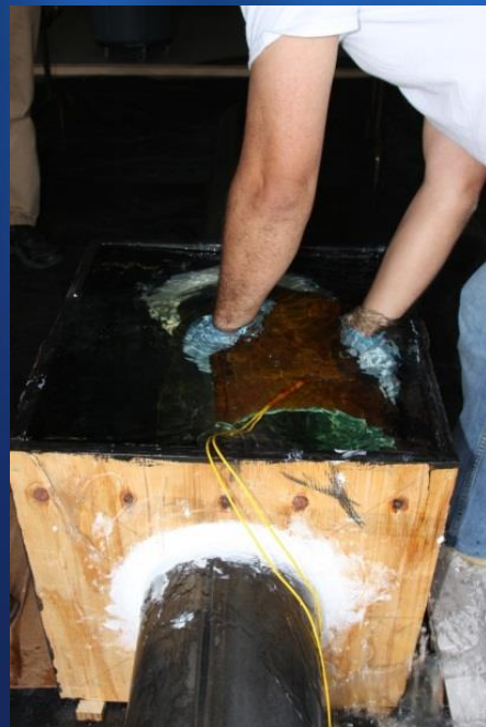
Adhesive Clamp Installation on 8-inch Test Pipe
