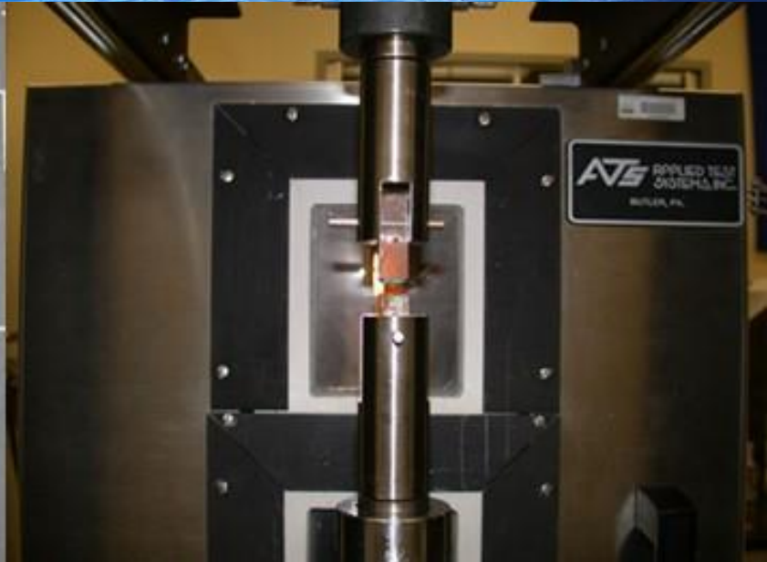
Test Article in Tensile Test Fixture
