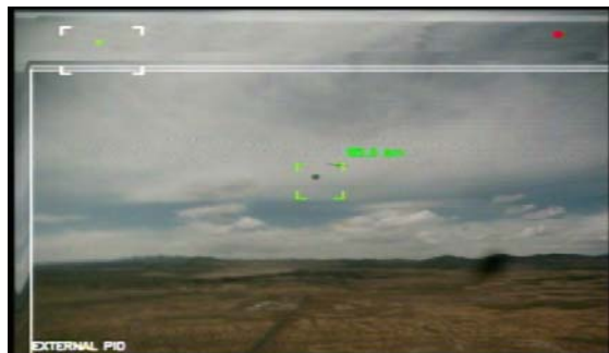
Figure 8 – A video frame from the seeker UAS camera showing the drogue and the user selected tracking point in the green box.
