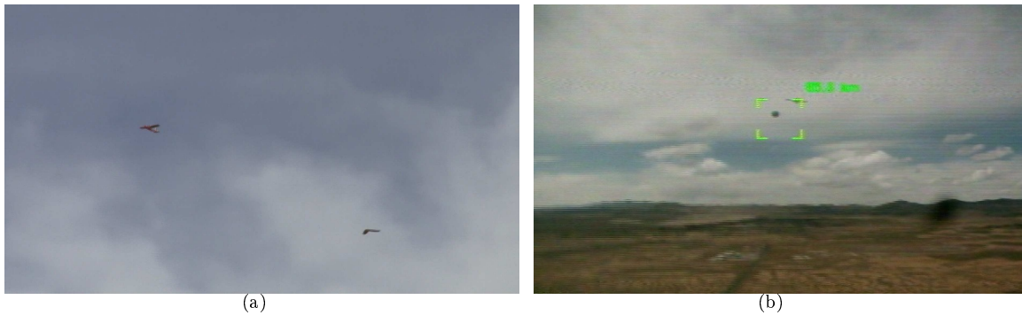
Fig. 11 (a) External video frame showing mothership and UAS in formation flight; (b) Single frame from UAS camera while following drogue. Drogue is visible in center of green acquisition box. Mothership is obscured by top right corner of acquisition box.
